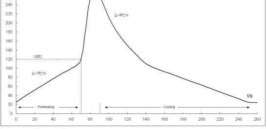
Fig2: Wave soldering profile
